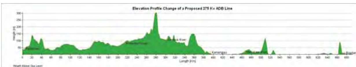
Figure A5.2 Elevation profile of a proposed 275 kV line from Pelaihari, Kalsel to Bontang Kaltim
